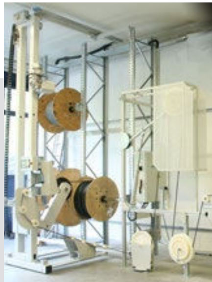
Cable rack with automated cable reel handling
