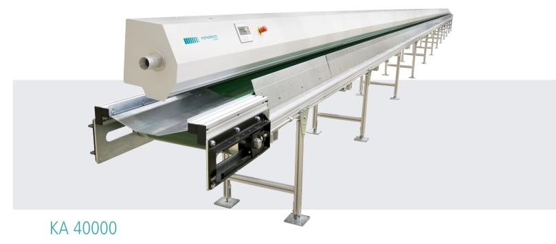
For flexible cable up to 35 mm. For lengths up to approx. 40 m.
